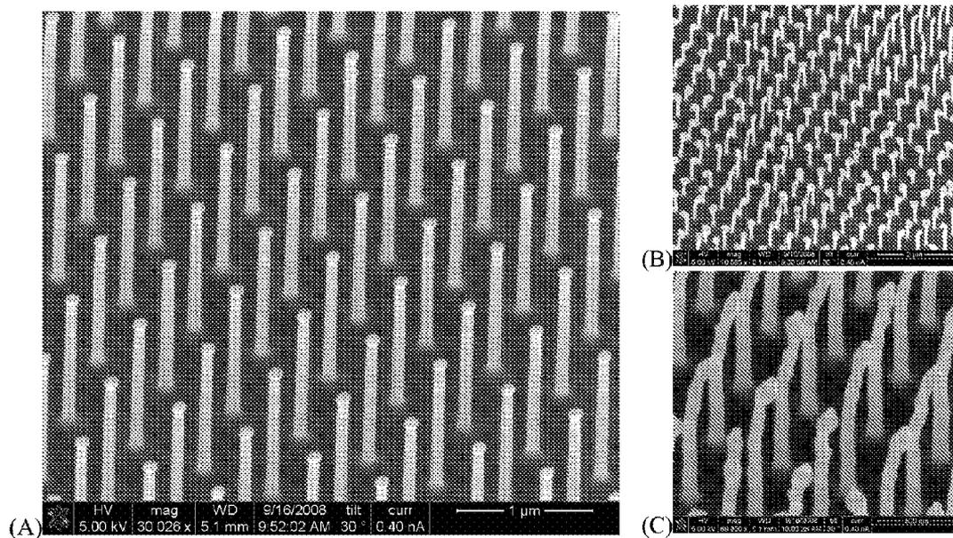
**Figure 7:** (A) Slender nanowires with 100 nm diameter before exposure to the desorption laser pulse. (B) and (C) Exposure of these thin posts to a high fluence desorption laser pulse results in the deformation of nanowires due to transient melting. Such melting and deformation was not observed for posts of larger diameter.
